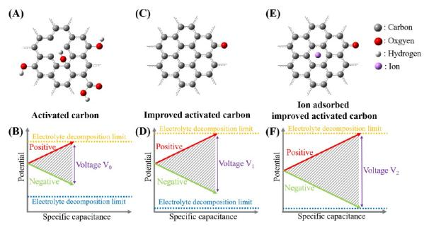
Figure 1. Approaches to widen supercapacitor operating voltage window by activated carbon modification
